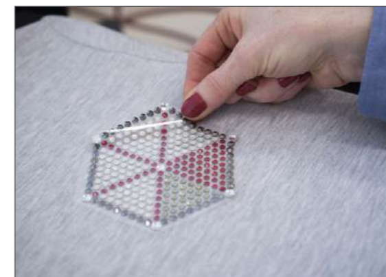
5 Place the transfer onto fabric where you want it to be applied (stones facing up).
