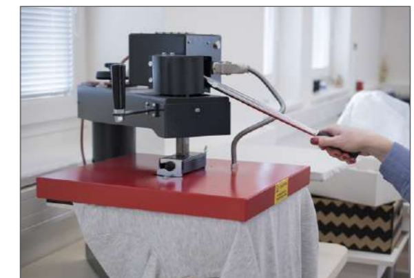
6 Press for 15-20 seconds with medium pressure and temperature at 160°C (make sure to cover the motif with a cotton cloth).
